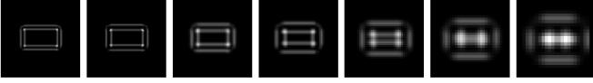
Fig. 4. An example of the set of 2D histograms, m_s , produced by the interest point detector when given a rectangle of edges weighted equally with unit motion. The scale, s , increases from left to right. Strong responses in the planes correspond with corners, parallel lines, and the ends of the rectangle.
