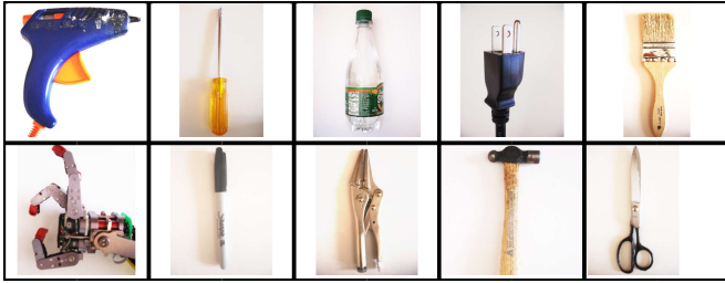
Fig. 2. We previously demonstrated the tip detection on these tools. (hot-glue gun, screwdriver, bottle, electrical plug, paint brush, robot finger, pen, pliers, hammer, and scissors). The method performed best on the tools with sharp tips.
