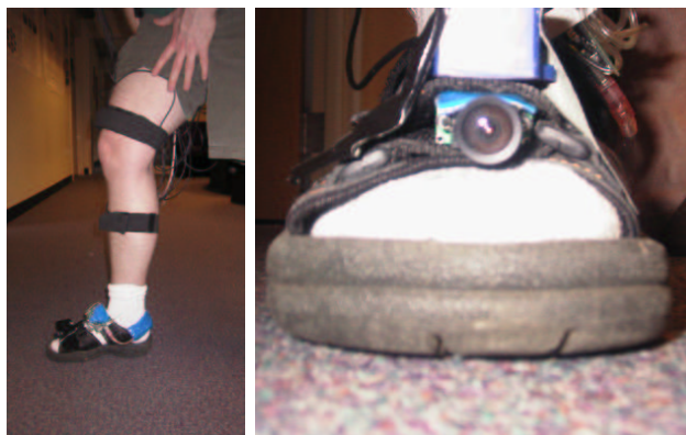
Figure 1. The system. A camera and inertial sensor are mounted on a sandal.
