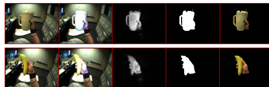
Figure 5: The wearable system currently achieves segmentation by active sensing. When the wearer brings an object up into view (first column), an oscillating light source is activated (second column). The difference between images (third column) is used to compute a mask (fourth column) and segment out the grasped object and the hand from the background via a simple threshold.(fifth column).
